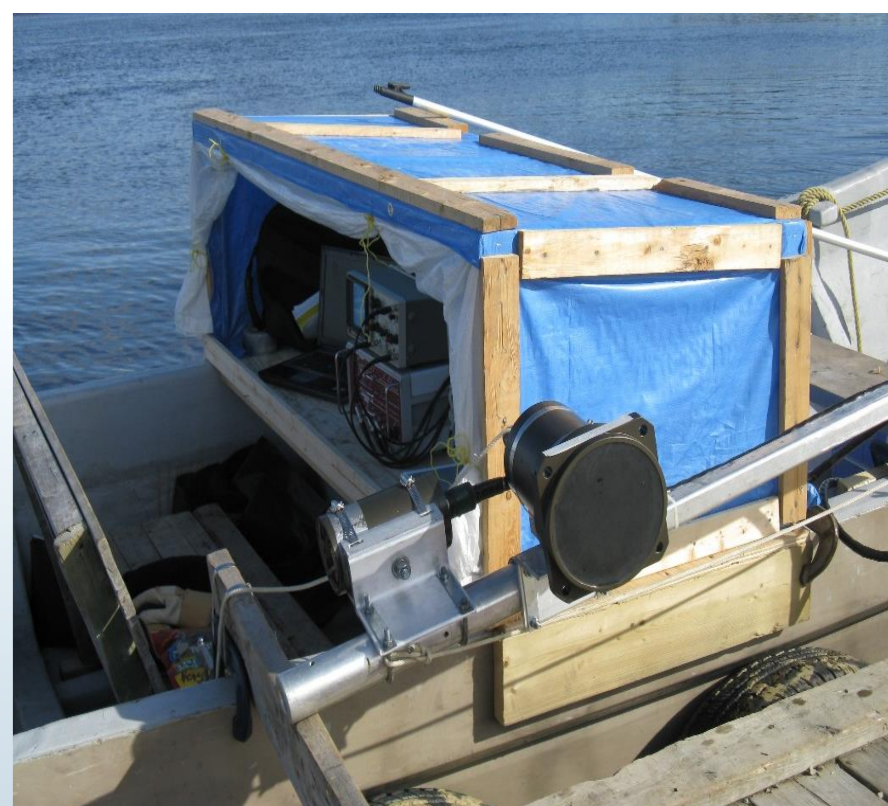
Figure 1. Mobile hydroacoustic sampling in shallow water.
